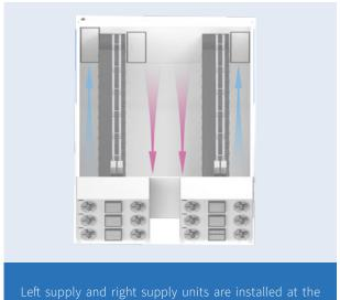
Left supply and right supply units are installed at the same end of Edge DC, hot/cold aisles containment can still be realized
